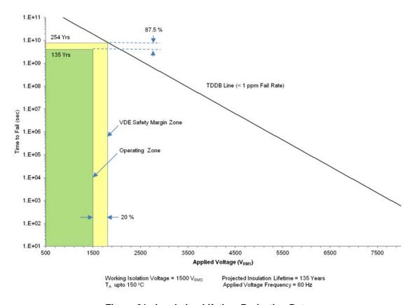
Figure 21. Insulation Lifetime Projection Data
