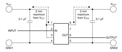
Figure 18. Typical ISO7710 Circuit Hook-up
