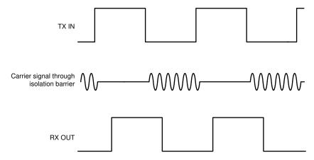
Figure 15. On-Off Keying (OOK) Based Modulation Scheme
