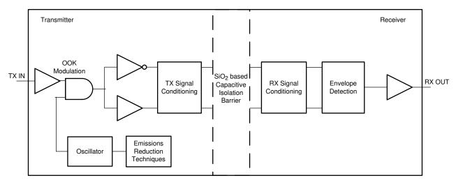
Figure 14. Conceptual Block Diagram of a Digital Capacitive Isolator
