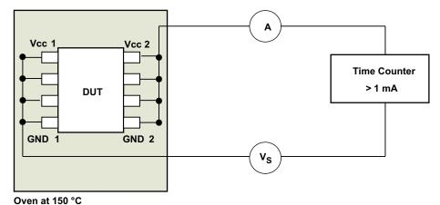
Figure 20. Test Setup for Insulation Lifetime Measurement
