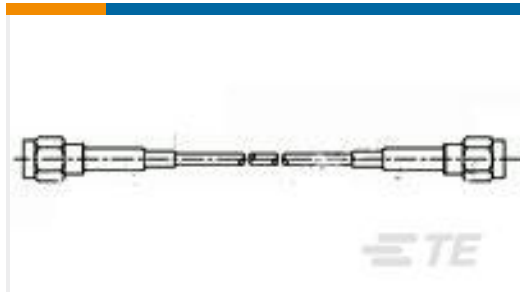
TE Part #1337808-3 50 OHM COAX SMA STR PLUG STR P
