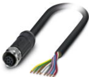
Sensor/Actuator cable, 8-position, PE-X halogen-free, black-gray RAL 7021, free cable end, on Socket straight M12, A-coded, Cable length: 10 m, for outdoor applications, With high-grade steel knurl
