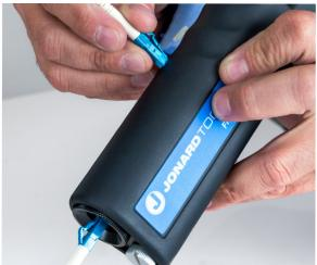
Fiber inspection microscopes have a focus wheel and features 2.5mm and 1.25mm adaters for use on most fiber connectors. The achromatic lens offers excellent imaging and intergrated laser filters for safety (not intented for use with illuminated imaging and integrated laser filters for safety (not intented for use with illuminated fibers) Coaxial illumination provides clear view of connector face and fiber.
