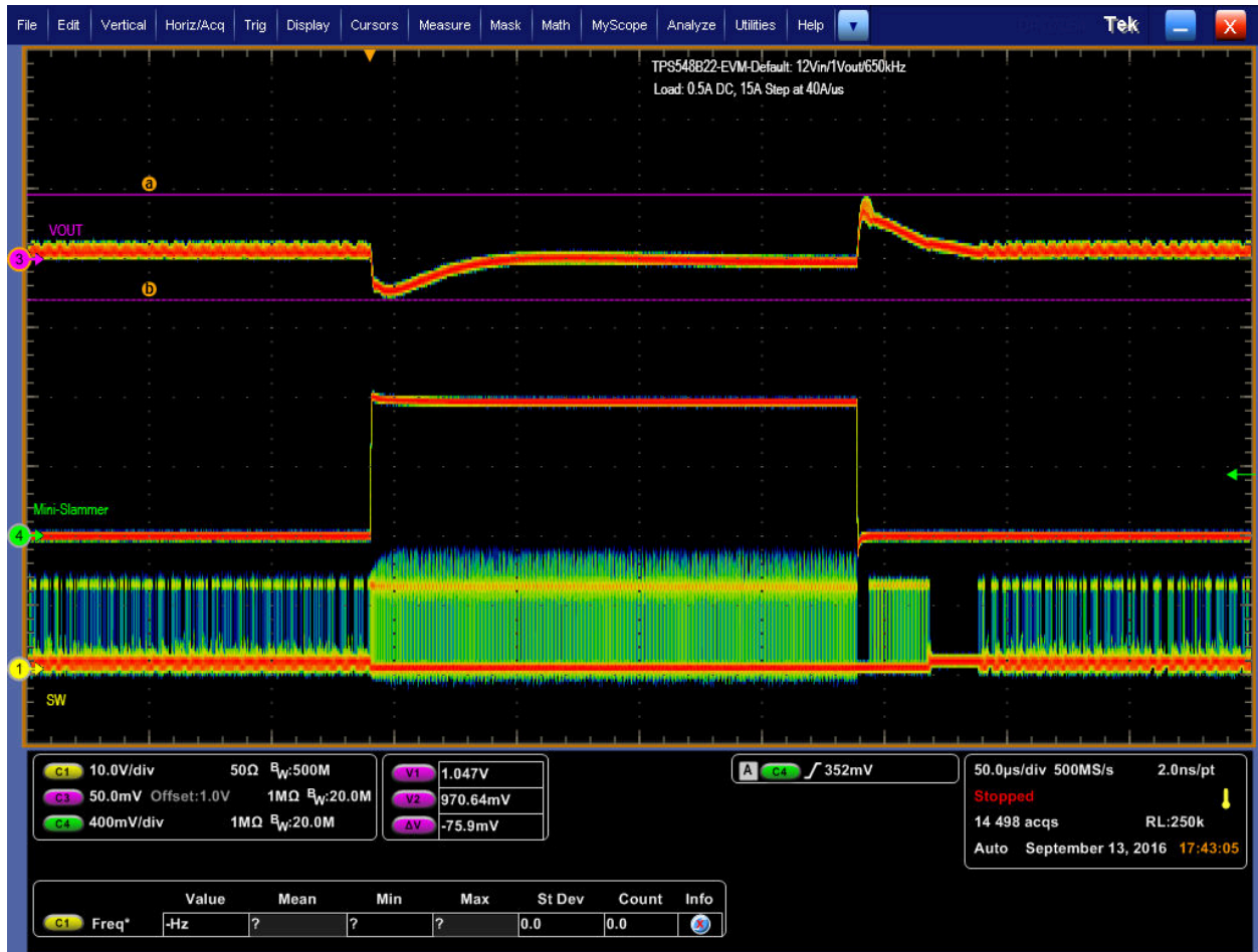
Figure 9-4. Transient Response of 1-V Output at 12 V IN , Transient is 0.5 A to 15.5 A, the Step is 15 A at 40 A/µs
