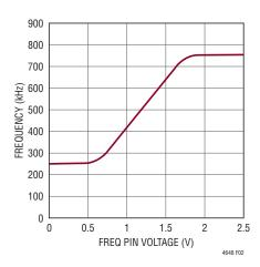
Figure 2. Operating Frequency vs FREQ Pin Voltage
