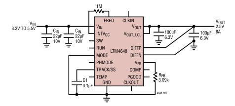
Figure 19. 3.3V to 5V  $V_{\text{IN}}$ , 2.5 $V_{\text{OUT}}$  at 8A Design with Increased 650kHz Frequency
