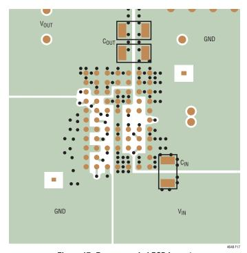
Figure 17. Recommended PCB Layout
