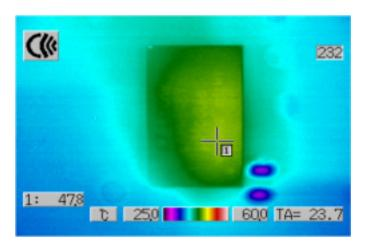
Figure 16. Thermal Image 5V<sub>IN</sub> to 1.5V<sub>OUT</sub> at 10A (No Heat Sink, No Air Flow and Room Temperature)
