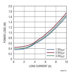
Figure 10. 5V<sub>IN</sub> to 3.3V<sub>OUT</sub>, 2.5V<sub>OUT</sub> and 1.5V<sub>OUT</sub> Power Loss
