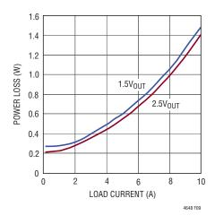
Figure 9. 3.3V<sub>IN</sub> to 2.5V<sub>OUT</sub> and 1.5V<sub>OUT</sub> Power Loss
