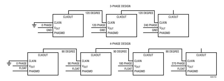
Figure 3. Examples of 3-Phase, 4-Phase Operation with PHASMD Table
