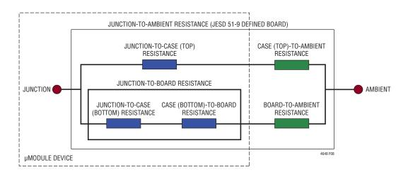
Figure 8. Graphical Representation of JESD51-12 Thermal Coefficients
