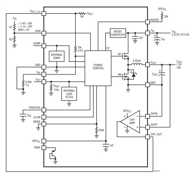
Figure 1. Simplified LTM4648 Block Diagram
