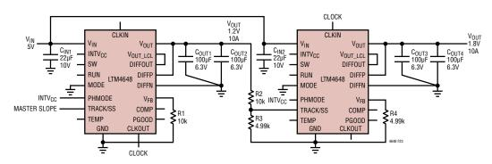
Figure 23. Dual Outputs 2-Phase LTM4648 Regulator with Tracking Function
