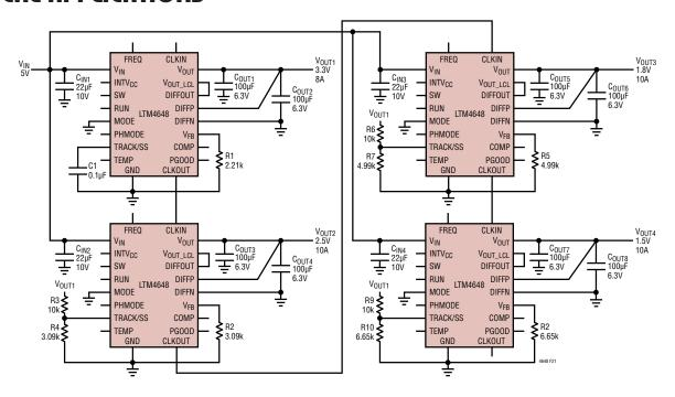
Figure 21. Quad Outputs 4-Phase LTM4648 Regulator with Tracking Function
