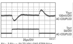
$5V_{IN}$ , 2.5 $V_{OUT}$ , 5A TO 10A LOAD STEP, 5A/ $\mu$ s  $C_{OUT}$  = 1 • 22 $\mu$ F, 6.3V, 1210 + 2 • 100 $\mu$ F 6.3V1210 CERAMIC CAPACITORS
