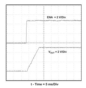
Figure 9. Start-Up Waveform, VOUT Relative to ENA
