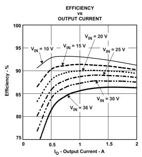
Figure 1. Measured Efficiency, TPS5420
