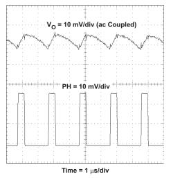
Figure 6. Measured Output Voltage Ripple, TPS5420
