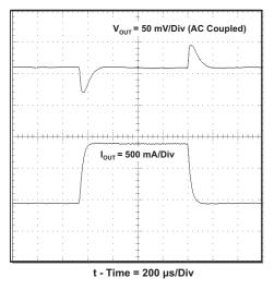
Figure 4. Load Transient Response, TPS5420
