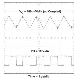
Figure 7. Input Voltage Ripple, TPS5420
