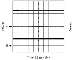
A: OUTPUT VOLTAGE:  $V_{OUT}$ ; 2V/DIV B: LOAD CURRENT:  $I_{LOAD}$  = 500 mA; 500 mA/DIV
