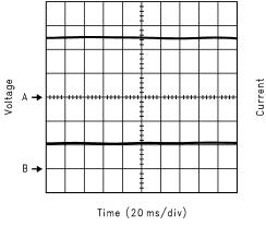
A: OUTPUT VOLTAGE: V<sub>OUT</sub>; 2V/DIV B: LOAD CURRENT: I<sub>LOAD</sub> = 500 mA; 500 mA/DIV
