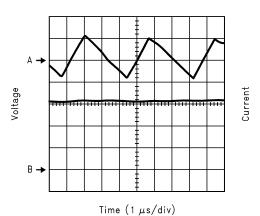
A: OUTPUT RIPPLE; 10 mV/DIV B: LOAD CURRENT: I<sub>LOAD</sub> = 3A; 1A/DIV
