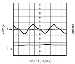
A: OUTPUT RIPPLE; 100 mV/DIV B: LOAD CURRENT: I<sub>LOAD</sub> = 500 mA; 1A/DIV
