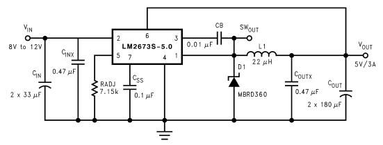
Figure 5. 5V/3A Design Circuit
