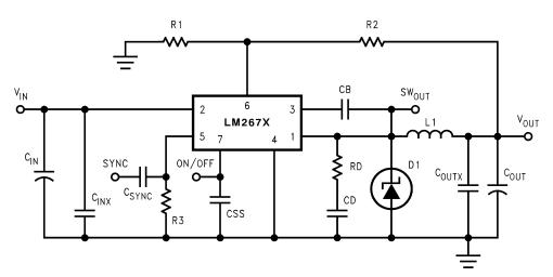
Figure 1. Example Schematic Showing Connection for all Components.
