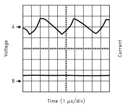
A: OUTPUT RIPPLE; 10 mV/DIV B: LOAD CURRENT: I<sub>LOAD</sub> = 0.5A; 1A/DIV
