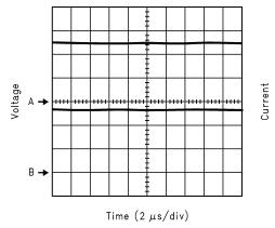
A: OUTPUT VOLTAGE: V<sub>OUT</sub>; 2V/DIV B: LOAD CURRENT: ILOAD = 2.5A; 1A/DIV
