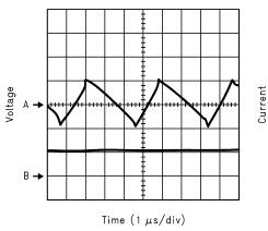
A: OUTPUT RIPPLE; 10 mV/DIV B: LOAD CURRENT: I<sub>LOAD</sub> = 1A; 1A/DIV
