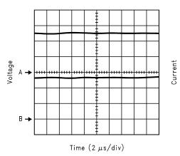
A: OUTPUT VOLTAGE: V<sub>OUT</sub>; 2V/DIV
