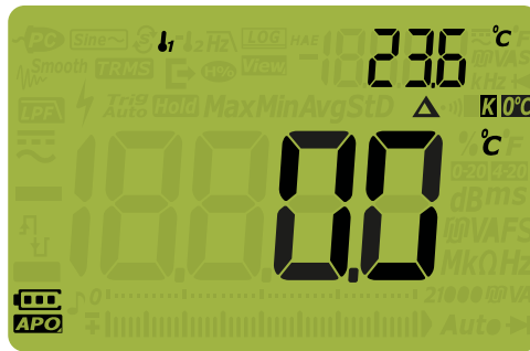
Figure 2-22 Temperature measurement without ambient compensation
