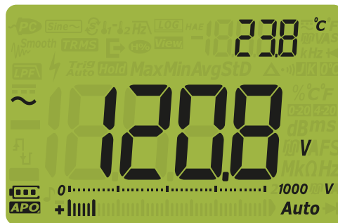
Figure 2-1 AC voltage display
