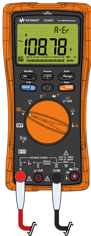
Figure 1-2 Example of wrong terminal input
