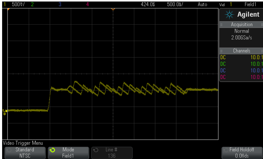
Figure 22 Triggering on Color Field 1 Alternating with Color Field 3
