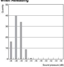
Sample: G5RL-1A-LN 12 VDC Number of relays: 100 pcs Range: A weighted sound pressure level, Fast, Max. hold Device connected to coil: Diode Testing environment:Room temperature and
