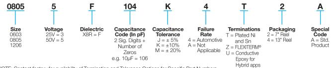
NOTE: Contact factory for availability of Termination and Tolerance Options for Specific Part Numbers.
