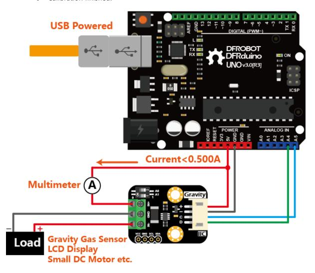
• The calibrated parameters "ina219Reading\_mA" and "extMeterReading\_mA" can now be used in this specific wattmeter module without recalibration for each measurement.
