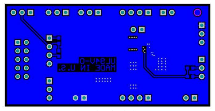
Figure 11. Bottom Layer Routing
