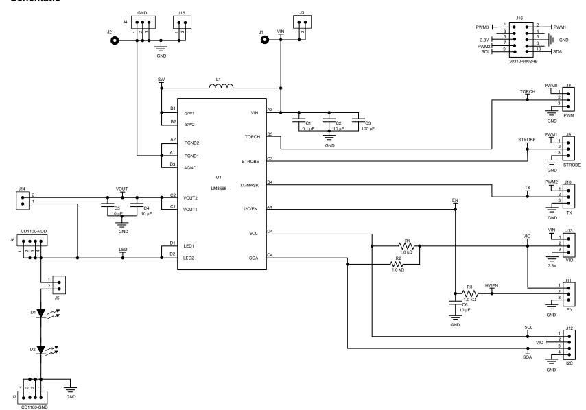
Figure 12. LM3565EVM Schematic
