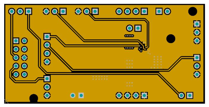
Figure 9. Middle Layer 1 Routing
