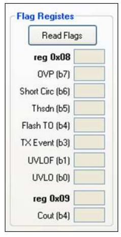
Figure 21. Fault Register
