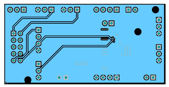
Figure 10. Middle Layer 2 Routing
