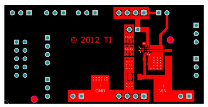
Figure 8. Top Layer Routing
