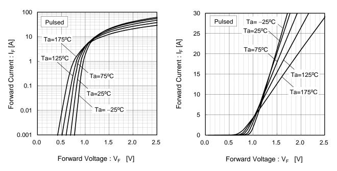
Fig.2  $V_F$  -  $I_F$  Characteristics
