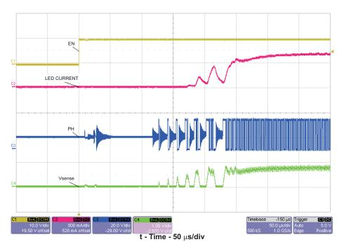
Figure 8. Start-up relative to EN, Vin=24V, lout=675mA
