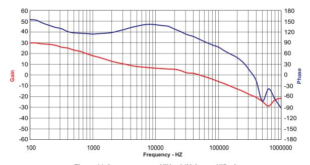
Figure 11. Loop response, VIN = 24V, lout = 675mA
