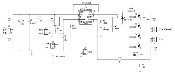
Figure 1. TPS54160EVM-535 Schematic Diagram
