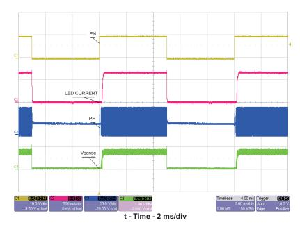
Figure 9. PWM Dimming, Vin=24V, Iout=675mA
