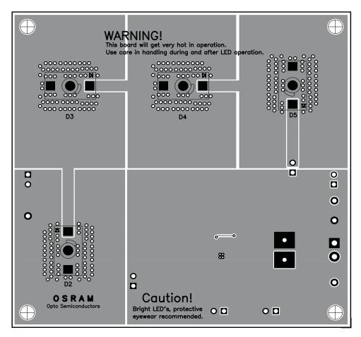
Figure 3. Bottom Assembly Layer
