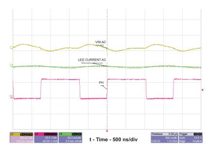
Figure 7. Input Voltage Ripple, Vin=24.0V, lout=675mA, AC Coupled
