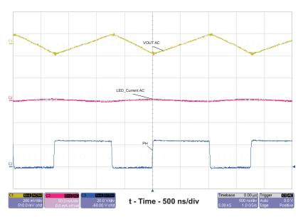
Figure 6. Output Ripple, Vin=24.0V, lout=675mA, AC Coupled
