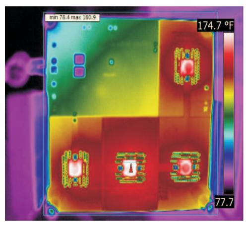
Figure 13. Thermal Performance, Bottom
