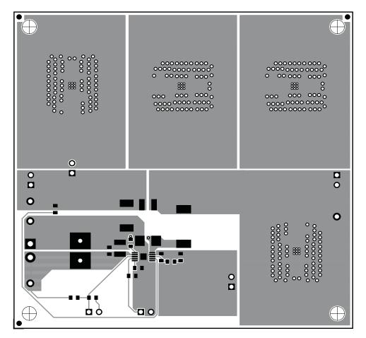
Figure 4. Top Layer Routing
