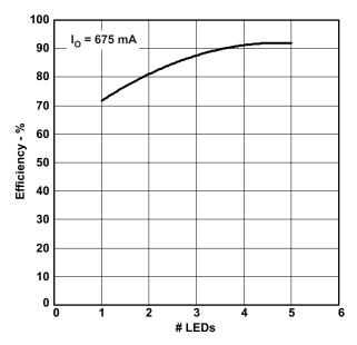
Figure 5. Efficiency, Vin=24V
