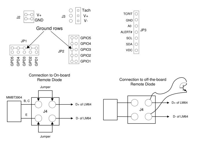
Figure 3. Header Connectors on the LM64 Evaluation Board
