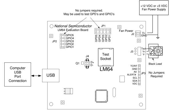
Figure 2. Test Setup using the LM64 Evaluation Board
