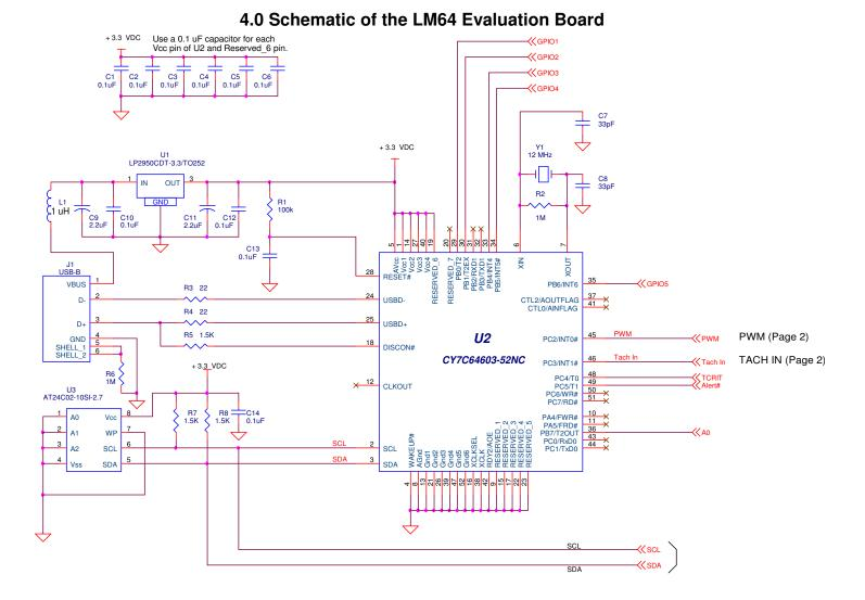
Figure 5a. LM64 Evaluation Board Schematic, Page 1 of 2
