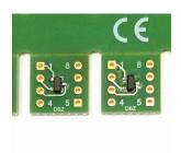
**Step 1:** Solder IC(s) to adapter PCB. Parts may be hand soldered or attached with IR or hot air reflow techniques.
