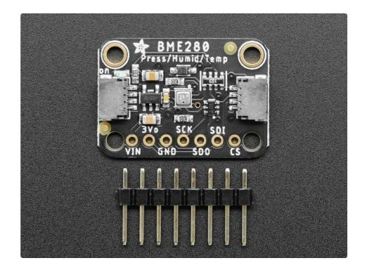
The BME280 is the next-generation of sensors from Bosch, and is the upgrade to the
