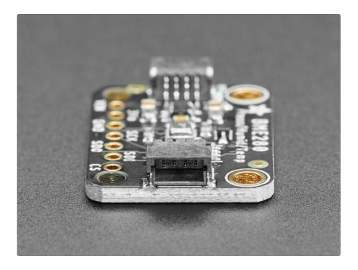
The breakout is made in the <u>STEMMA QT form factor</u> (https://adafru.it/LBQ), making them easy to interface with. The <u>STEMMA QT connectors</u> (https://adafru.it/JqB) on either side are compatible with the <u>SparkFun Qwiic</u> (https://adafru.it/Fpw) I2C connectors. This allows you to make solderless connections between your development board and the BME280 or to chain it with a wide range of other sensors and accessories using a <u>compatible cable</u> (https://adafru.it/JnB).
