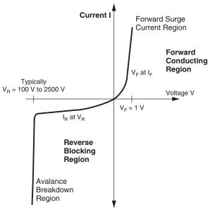
Fig. 1 - Basic Rectifier Characteristics
