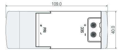
wire stripping length: 6-7mm recommended tightening torque: 0.25Nm tc= case temperature measuring point FC= fixing centers
