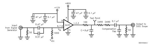
Note: 8 pF load includes parasitic capacitance.
