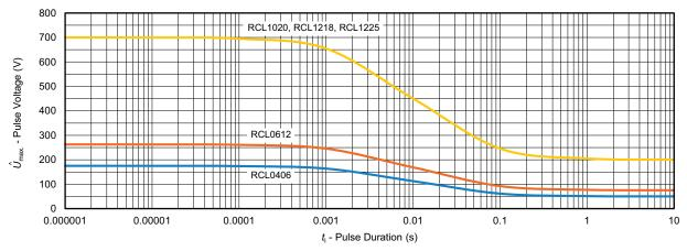
Maximum pulse voltage, single and continuous pulses; applicable if  $\dot{P} \leq \dot{P}_{max}$ ; for permissible resistance change equivalent to 8000 h operation
