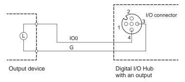
The output power that provides load current is supplied from the IO-Link Master Unit through the IO-Link cable to the Digital I/O Hub.
