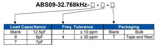
\*Contact ABRACON for non-standard load capacitance
