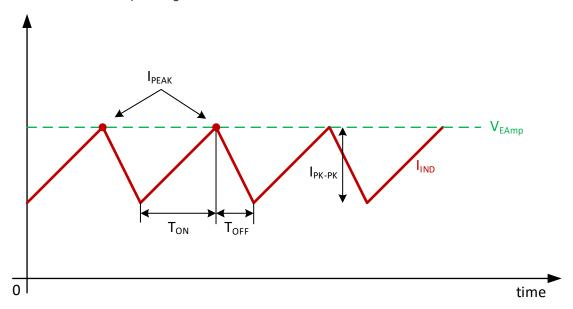
Figure 7. Peak-Current Architecture Operation
