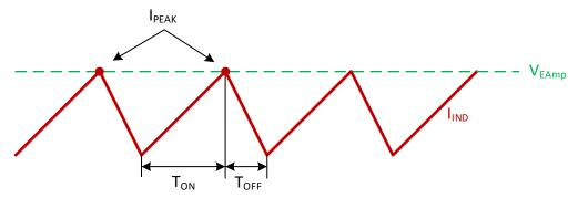
Figure 11. Peak-Current Buck Operation
