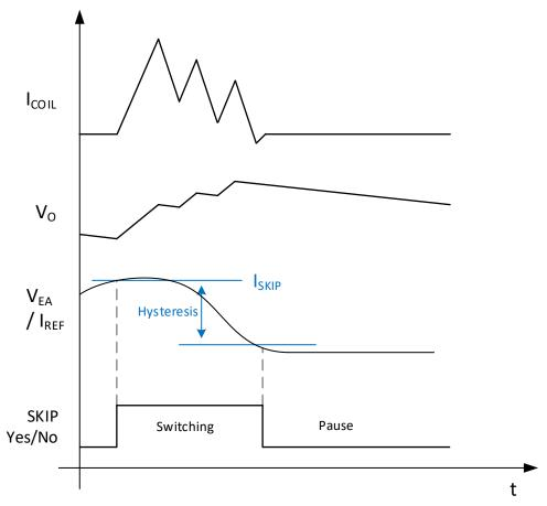
Figure 12. Power Safe Mode Operation Curves
