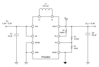
Figure 13. 3.3 V<sub>OUT</sub> Typical Application
