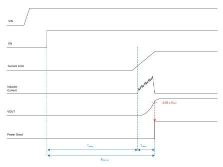
Figure 6. Device Start-up Scheme
