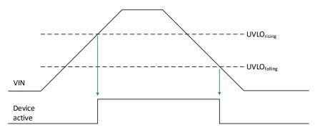
Figure 5. Rising and Falling Undervoltage Lockout Behavior
