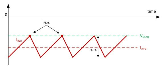
Figure 8. Peak-Current Operation, Reverse Current
