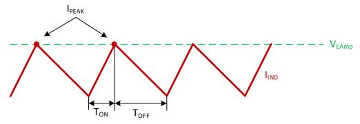
Figure 9. Peak-Current Boost Operation
