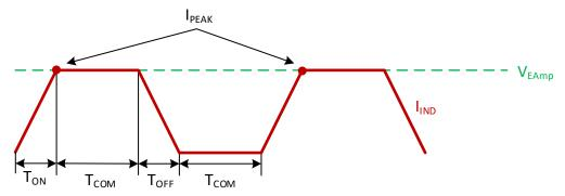
Figure 10. Peak-Current Buck-Boost Operation
