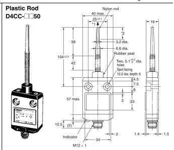
\*1. Operation is possible in any direction except parallel to the axis **4**.
