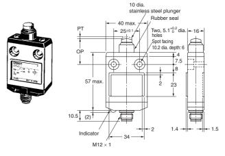
Note: Unless otherwise specified, a tolerance of  $\pm 0.4 \ \text{mm}$  applies to all dimensions.
