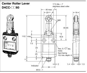
Note: Unless otherwise specified, a tolerance of  $\pm 0.4 \ \text{mm}$  applies to all dimensions.
