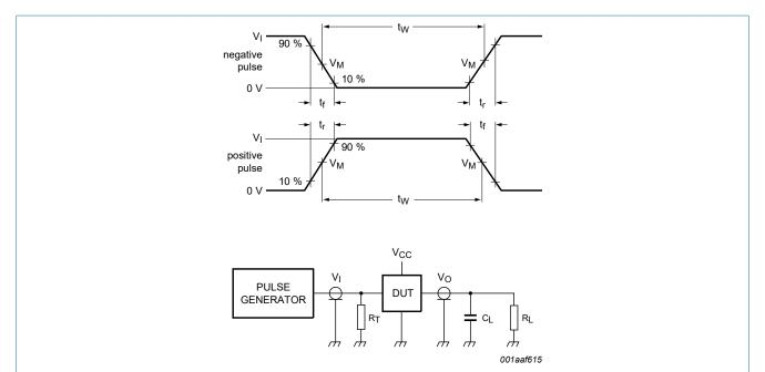
Test data is given in <u>Table 9</u>. Definitions for test circuit:
