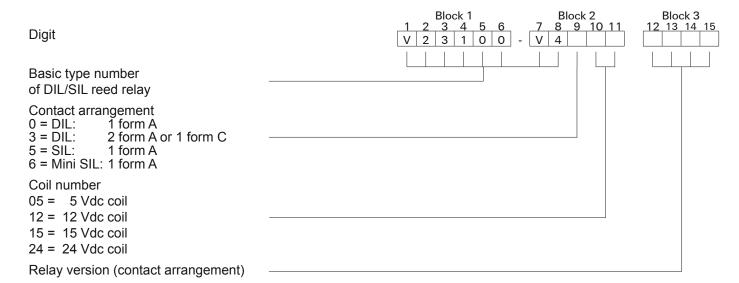
Ordering example: V23100-V4005-A010 DIL reed relay with 1 make, 5 V nominal voltage, with clamping diode (spark suppression)
