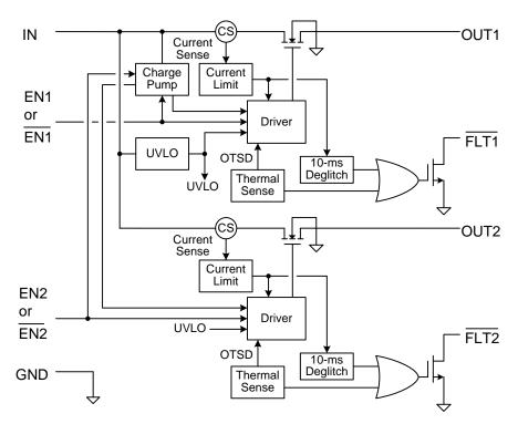
Figure 30. TPS20xxC-2 Functional Block Diagram
