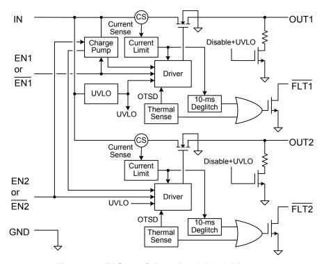
Figure 29. TPS20xxC Functional Block Diagram
