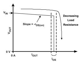
Figure 28. Output Characteristic Showing Current Limit
