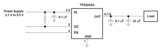
Figure 24. Typical Application (Example, TPS2045A)
