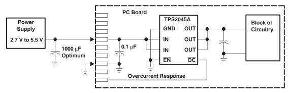
Figure 31. Typical Hot-Plug Implementation (Example, TPS2045A)
