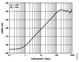
Figure 37. Common-Mode Rejection Ratio (CMRR) vs. Frequency
