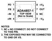
Figure 5. 8-Lead LFCSP Pin Configuration
