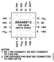
Figure 7. 16-Lead LFCSP Pin Configuration
