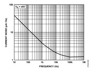
Figure 38. Input Current Noise vs. Frequency
