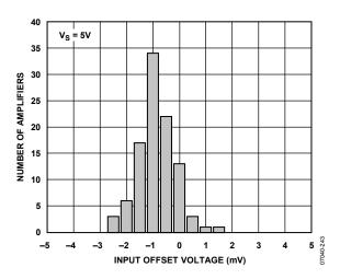
Figure 43. Input Offset Voltage Distribution,  $V_s = 5 V$
