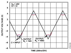
Figure 36. Output Overdrive Recovery for Various Resistive Loads
