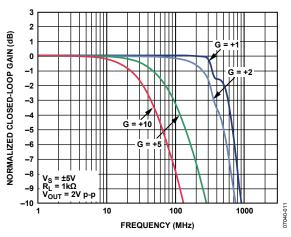
Figure 11. Large Signal Frequency Responses for Various Gains (LFCSP)
