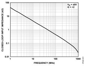
Figure 31. Closed-Loop Input Impedance vs. Frequency
