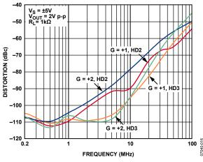
Figure 16. Harmonic Distortion vs. Frequency and Gain (LFCSP)
