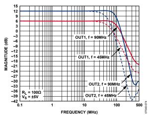
Figure 55. Low-Pass Filter Response
