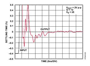
Figure 23. Short-Term Settling Time (LFCSP)
