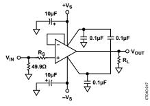
Figure 49. Noninverting Load Configuration
