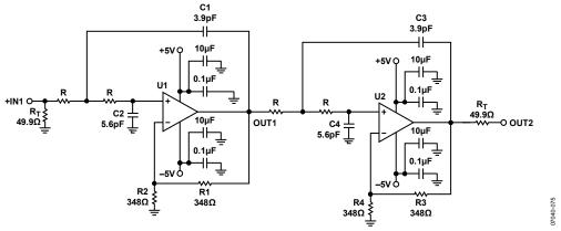
Figure 56. 4-Pole, Sallen-Key Low-Pass Filter (ADA4857-2)
