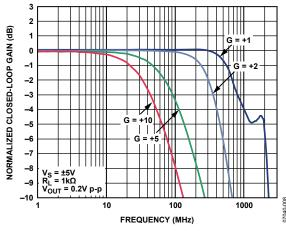
Figure 8. Small Signal Frequency Responses for Various Gains (LFCSP)
