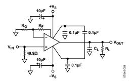
Figure 51. Typical Capacitive Load Configuration (LFCSP)
