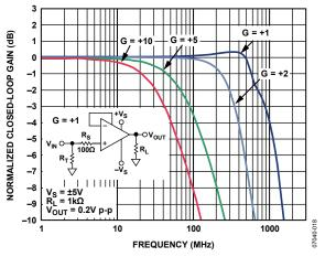
Figure 18. Small Signal Frequency Response for Various Gains (SOIC),  $R_{\rm S}$  = 100  $\Omega$  for G = +1
