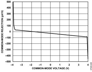
Figure 46. Common-Mode Rejection vs. Common-Mode Voltage
