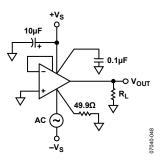
Figure 53. Negative Power Supply Rejection
