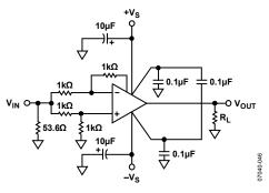
Figure 52. Common-Mode Rejection
