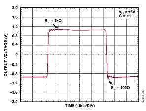
Figure 30. Large Signal Transient Response for Various Load Resistances (LFCSP)
