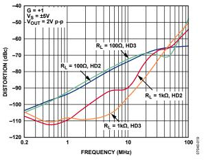
Figure 19. Harmonic Distortion vs. Frequency and Load (LFCSP)
