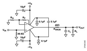
Figure 54. Typical Capacitive Load Configuration (SOIC)
