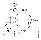
Figure 50. Positive Power Supply Rejection
