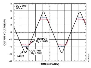
Figure 33. Input Overdrive Recovery for Various Resistive Loads
