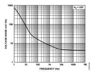
Figure 41. Input Voltage Noise vs. Frequency
