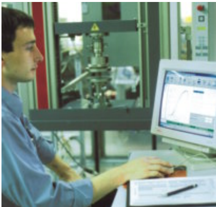
Testing the properties of polymer bearings
