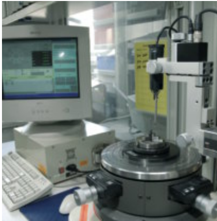
Measurement of the inner diameter of a pressfit plain bearing
