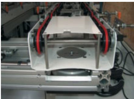
Handling- and transportsystem for Semiconductor-Carrier/-Box. The complete system is suitable for the use in cleanrooms, lubrication- and maintenance-free
