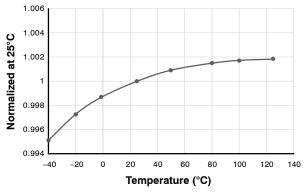
Figure 8.  $V_{CS(LIM-MIN)}$  vs. Temperature
