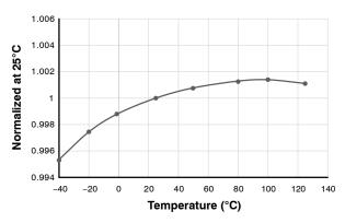
Figure 5. V<sub>DIM(MAX)</sub> vs. Temperature
