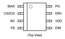
Figure 3. Pin Configuration
