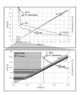
Figure 12. NCL35076 Dimming Curve and CC Tolerance
