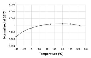
Figure 4. V<sub>BIAS</sub> vs. Temperature
