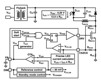
Figure 10. NCL35076 Block Diagram
