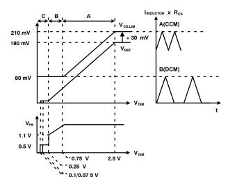
Figure 11. Operation Mode vs. V<sub>DIM</sub>
