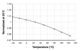
Figure 6.  $g_{M(FB)}$  vs. Temperature
