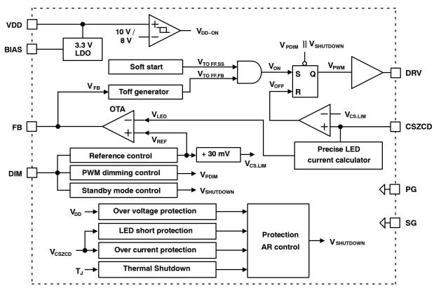
Figure 2. Simplified Block Diagram
