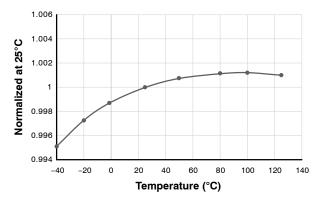
Figure 9. V<sub>DD(OVP)</sub> vs. Temperature
