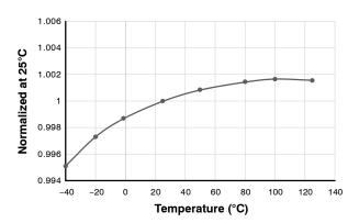
Figure 7.  $V_{CS(REG-MAX)}$  vs. Temperature
