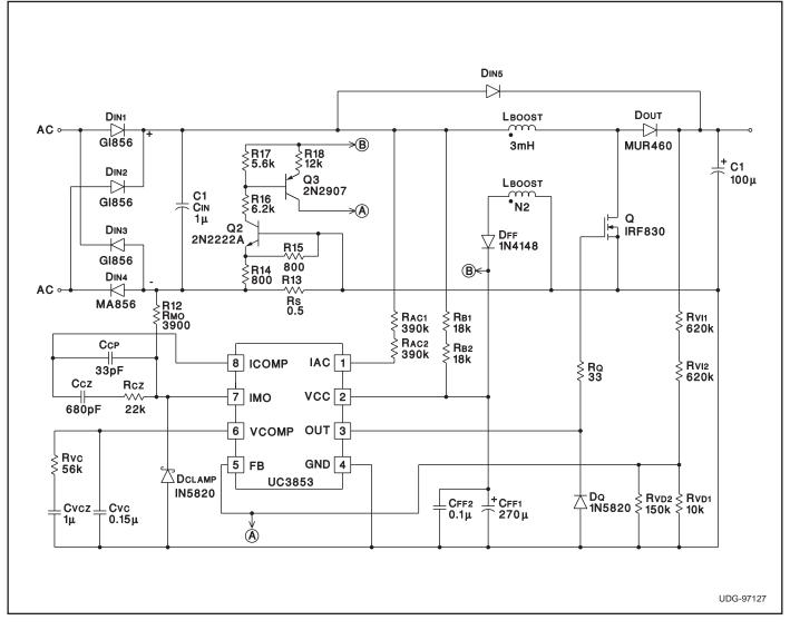
Note: the application circuit shown is a 100W, 75KHz design. Additional application information can be found in Application Note U–159 and Design Note DN–78.
