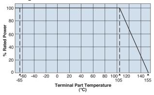
For resistors operated at an ambient temperature of  $105^{\circ}$ C or above, a power rating shall be derated in accordance with the above derating curve.
