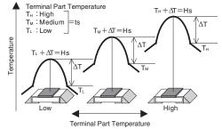
The temperature of the resistor will increase the same △T from the standard terminal part temperature regardlless of the ambient temperature when the same power is applied. This is because there is hardly any heat dissipation from the resistor surface to the ambient air.
