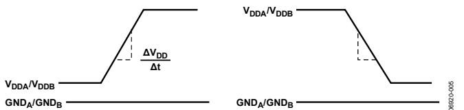
Figure 14. Transient Immunity Waveforms, Output Supplies
