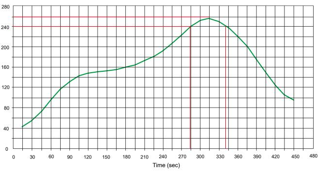
Peak Temp=257°C, Ramp Rate=0.802deg. °C/sec
