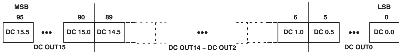
Figure 14. Dot Correction Data Packet Format
