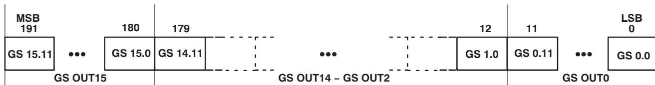
Figure 18. Grayscale Data Packet Format
