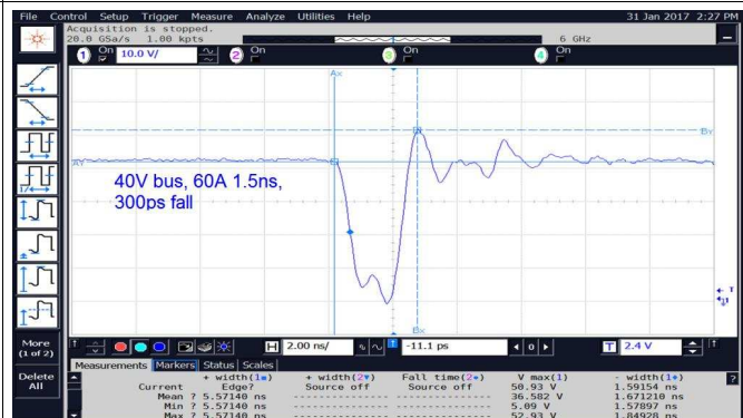
Figure 14. V_{DS} for 1.5 ns Pulse With 40V of Bus Voltage
