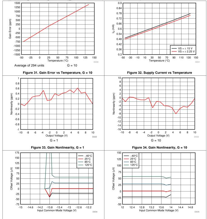
Figure 35. Offset Voltage vs Negative Common-Mode
