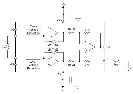
Figure 65. Parasitic Resistance Shown at the Reference Pin
