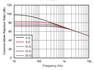
Figure 66. The Effect of Increasing Resistance at the Reference Pin
