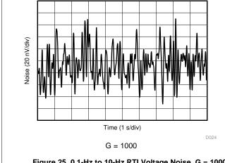
Figure 25. 0.1-Hz to 10-Hz RTI Voltage Noise, G = 1000
