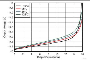
Figure 37. Positive Output Voltage Swing vs Output Current
