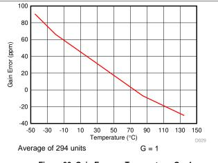
Figure 30. Gain Error vs Temperature, G = 1
