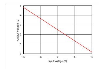
Figure 70. PLC Output Voltage vs Input Voltage
