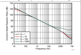
Figure 17. CMRR vs Frequency (RTI)
