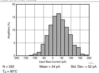
Figure 8. Typical Distribution of Input Bias Current,  $T_A = 90^{\circ}C$
