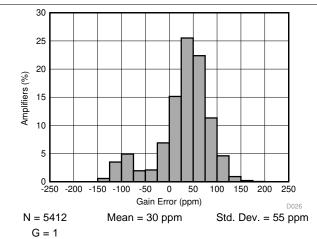
Figure 27. Typical Distribution of Gain Error, G = 1
