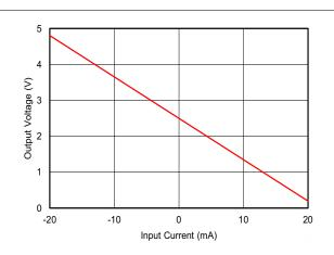
Figure 71. PLC Output Voltage vs Input Current
