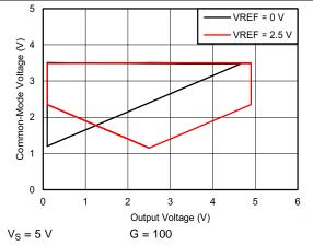
Figure 51. Input Common-Mode Voltage vs Output Voltage
