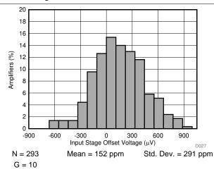
Figure 28. Typical Distribution of Gain Error, G = 10
