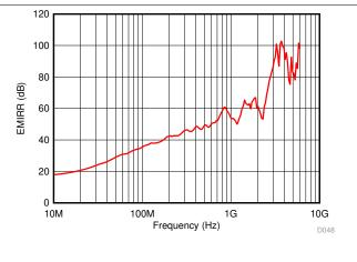
Figure 57. Differential-Mode EMIRR Testing
