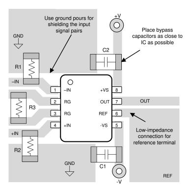
Figure 75. Example Schematic and Associated PCB Layout
