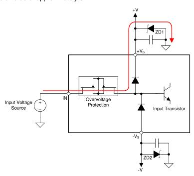
Figure 62. Input Current Path During an Overvoltage Condition
