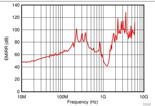
Figure 49. Differential-Mode EMI Rejection Ratio
