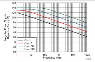
Figure 20. Negative PSRR vs Frequency (RTI)
