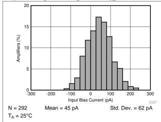
Figure 7. Typical Distribution of Input Bias Current,  $T_A = 25^{\circ} \text{C}$
