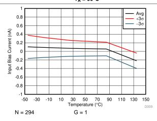
Figure 10. Input Bias Current vs Temperature
