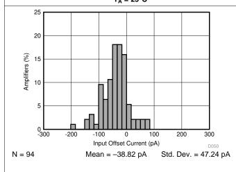
Figure 9. Typical Distribution of Input Offset Current
