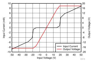
Figure 63. Input Current vs Input Overvoltage
