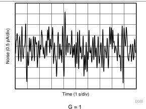
Figure 26. 0.1-Hz to 10-Hz RTI Current Noise
