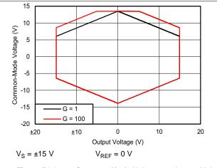
Figure 53. Input Common-Mode Voltage vs Output Voltage
