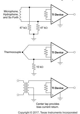
Figure 68. Providing an Input Common-Mode Current Path
