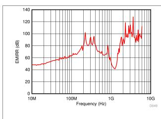
Figure 56. Common-Mode EMIRR Testing
