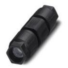
QUICKON cable connector, black, 3+PE-pos., 0.75 mm<sup>2</sup> ... 1.5 mm<sup>2</sup> /500 V/15 A, for a cable diameter of 6 mm ... 12 mm.
