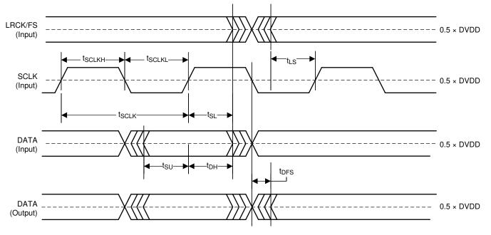
Figure 7-1. Serial Audio Port Timing in Slave Mode
