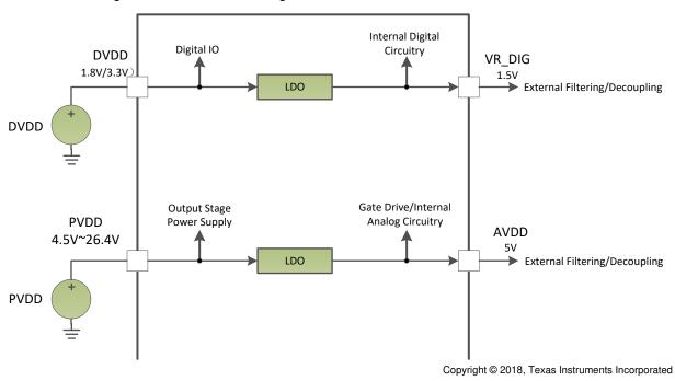
Figure 9-1. Power Supply Function Block Diagram
