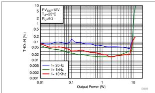
Figure 8-3. THD+N vs Frequency (Ferrite bead as Output Filter, BD Modulation, BTL Mode)
