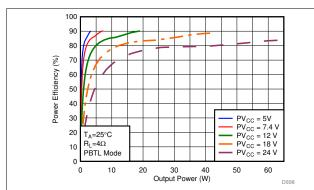
Figure 8-10. Efficiency vs Output Power (Inductor as Output Filter, Hybrid modulation, PBTL mode)
