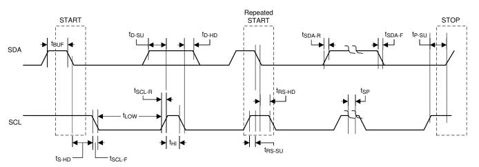
Figure 7-2. I<sup>2</sup>C Communication Port Timing Diagram
