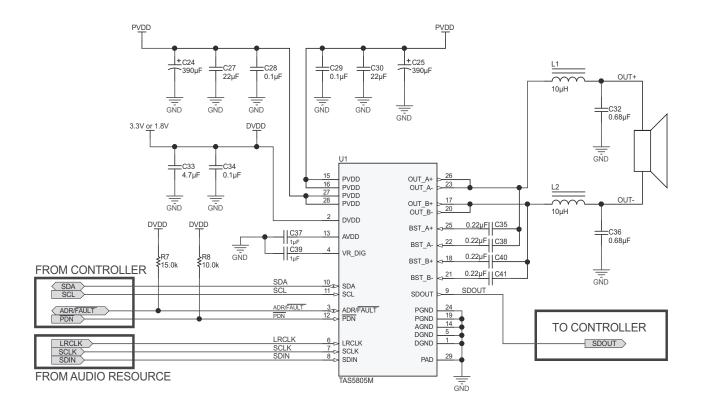
Figure 8-9. Mono (PBTL) System Application Schematic
