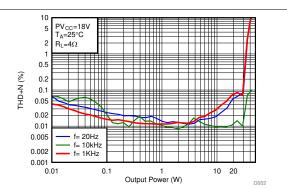
Figure 8-11. THD+N vs Output Power (Inductor as Output Filter, Hybrid Modulation, PBTL mode)
