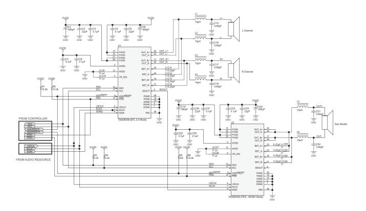
Figure 8-12. 2.1 (2.1 CH with Two TAS5805M Devices) Application Schematic
