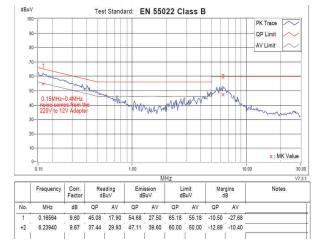
Figure 8-5. Conducted Emission with Ferrite Bead Filter - Line
