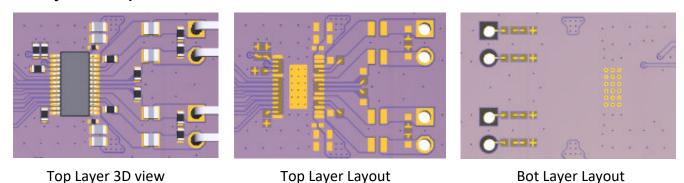
Figure 9-1. 2.0 (Stereo BTL with Ferrite Bead as Output Filter) Layout View
