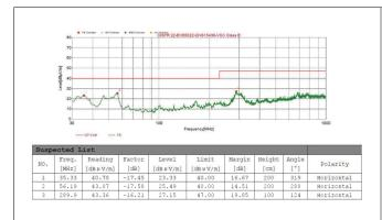
Figure 8-7. Radiated Emission with Ferrite Bead Filter - Horizontal
