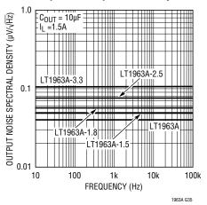
LT1963A-3.3 10Hz to 100kHz Output Noise
