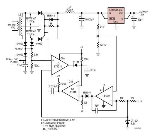
SCR Pre-Regulator Provides Efficiency Over Line Variations
