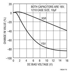
Figure 10. Ceramic Capacitor DC Bias Characteristics
