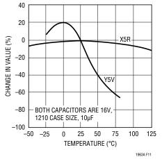
Figure 11. Ceramic Capacitor Temperature Characteristics
