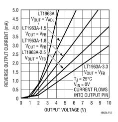
Figure 12. Reverse Output Current
