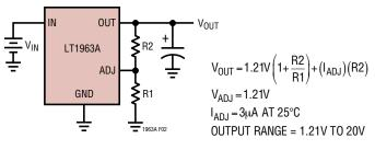
Figure 2. Adjustable Operation
