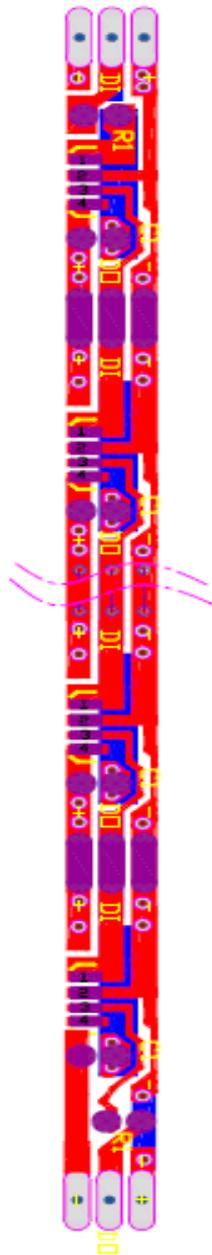
Product signal input and output must be connected in series Protection resistor R1, R1 depends on the size of the cascade lamp beads, the greater the number of cascade, the smaller R1, the general recommended value between 200-2K $\Omega$ , usually recommended Worth about 500  $\Omega$  euros;
