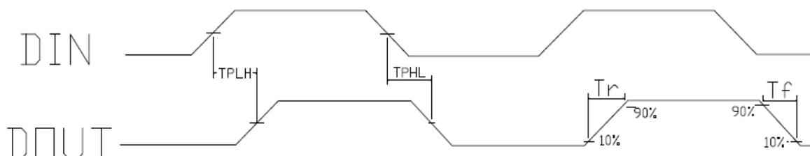
**12. The data transmission time ( $T_H+T_L=1.25\mu s\pm 600ns$ ):**
