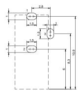
General tolerance ±0.05 Do not use shunt terminal for power supply. Purpose of terminals 2 & 3 is only plug in / plug out detection
