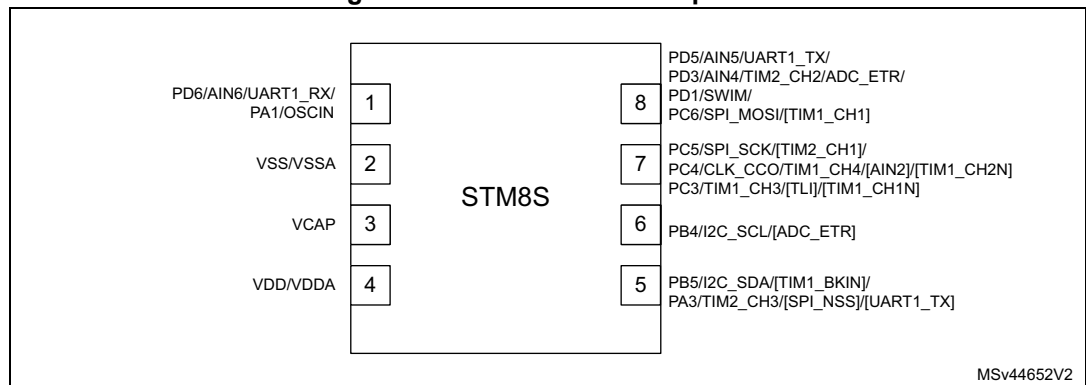
Figure 3. STM8S001J3 SO8N pinout
