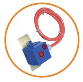
The FCTE is a heat sensor, which is attached to the outlet pipe from a pump. This device works by reacting to the temperature at the outlet of any centrifugal type pump, which will rapidly rise past  $45^{\circ}$  if the inlet water level falls below the centre line of the inlet. The unit will cut off the electrical supply to the pump, so protecting it from damage. Manual resetting of this unit allows the pump to restart.
