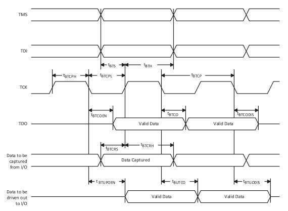
Figure 3.6. JTAG Port Timing Waveforms
