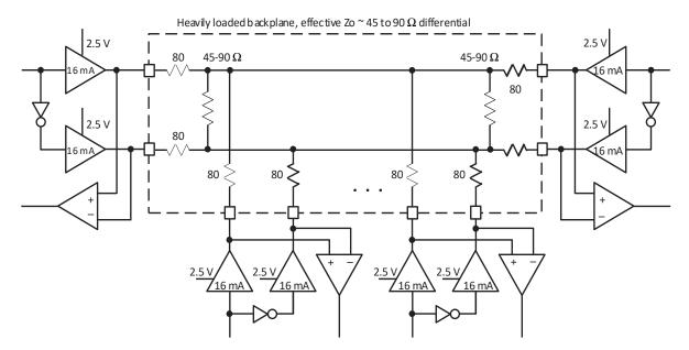
Figure 3.2. BLVDS Multi-point-Output Example
