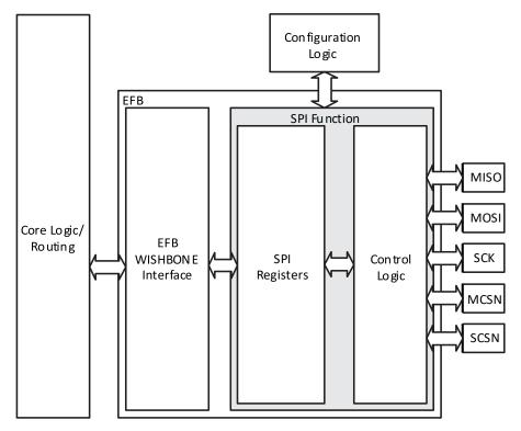
Figure 2.18. SPI Core Block Diagram
