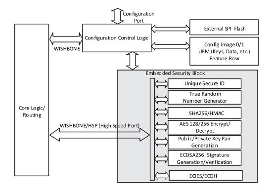
Figure 2.16. ESB Core Block Diagram
