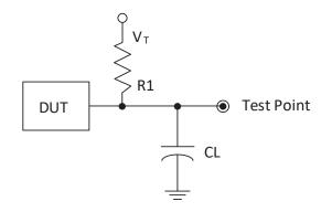
Figure 3.7. Output Test Load, LVTTL and LVCMOS Standards
