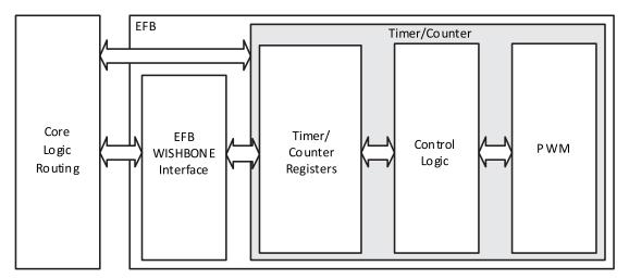
Figure 2.19. Timer/Counter Block Diagram
