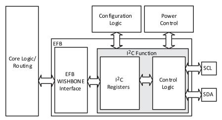
Figure 2.17. I<sup>2</sup>C Core Block Diagram
