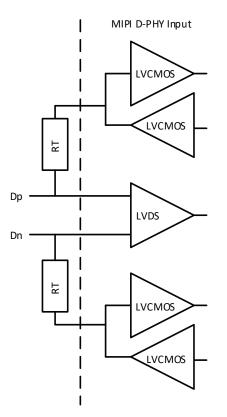
Figure 3.4. MIPI D-PHY Input Using External Resistors
