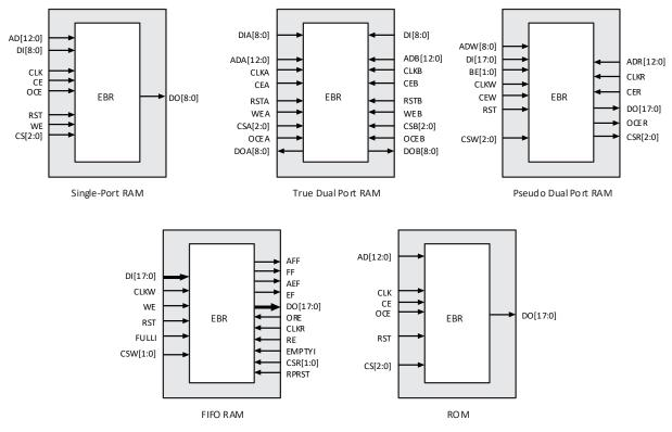
Figure 2.7. sysMEM Memory Primitives
