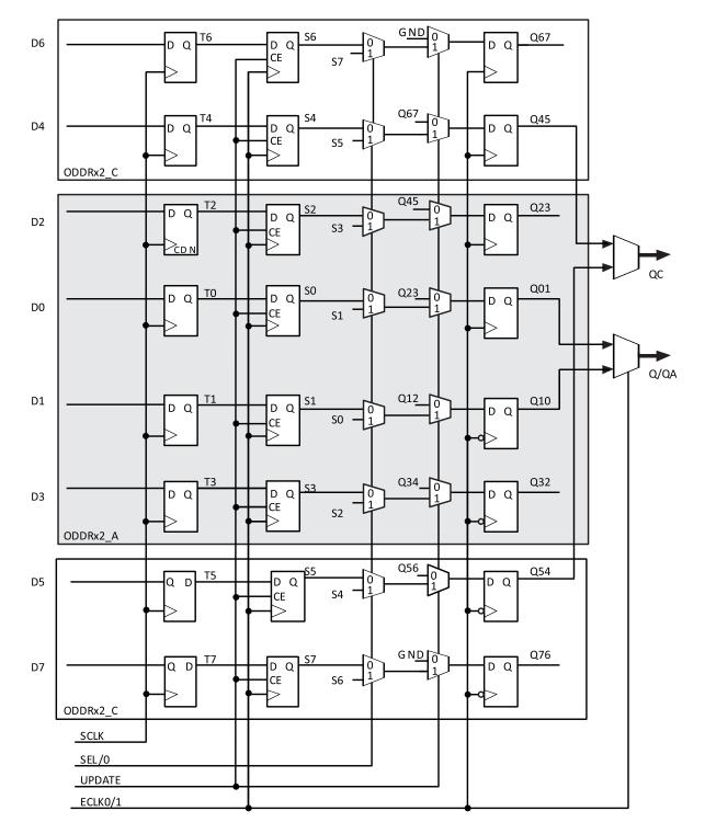
Figure 2.13. Output Gearbox
