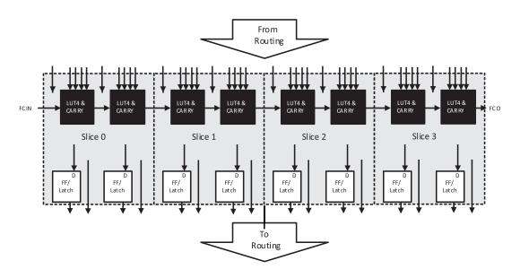
Figure 2.2. PFU Block Diagram
