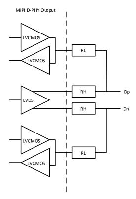
Figure 3.5. MIPI D-PHY Output Using External Resistors
