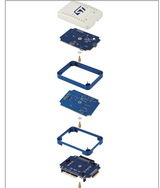
Figure 17. Opened casing for access to all connectors with B-STLINK-VOLT
