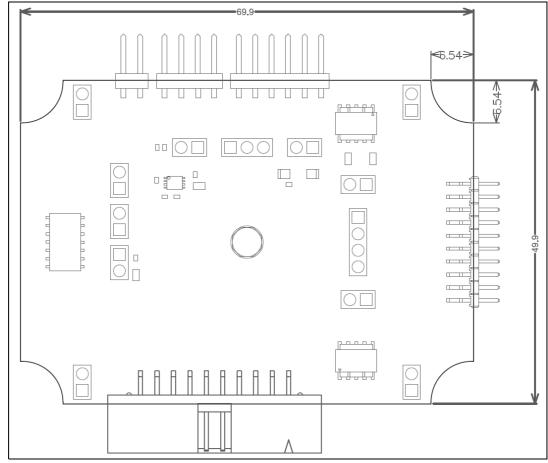
Figure 12. MB1440 mechanical drawing
