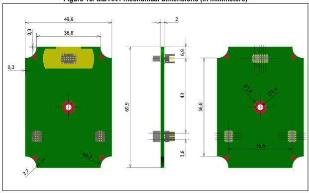
Figure 15. MB1441 mechanical dimensions (in millimeters)
