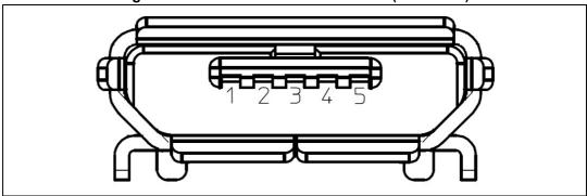
Figure 14. USB Micro-B connector CN5 (front view)
